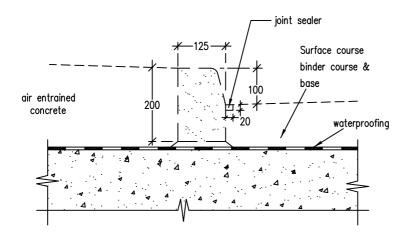
PRECAST CONCRETE ROAD KERB 125mmx200mm HALF BATTER PATTERN DETAIL ON STRUCTURE
