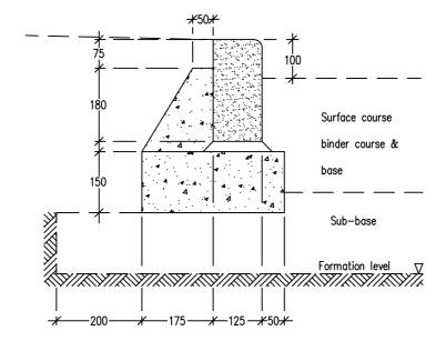
PRECAST CONCRETE ROAD KERB 125mm x 255mm BULLNOSE PATTERN DATE: Mar 2013
